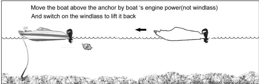
NOTE: The windlass is designed to lift the anchor, rather than to drag the boat or for mooring.
