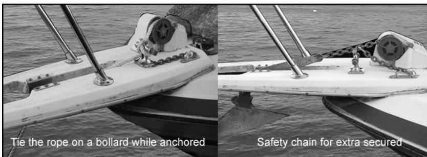
8. The anchor windlass is not designed for continuous operation. Do not use for more than **15 minutes** at a time under loading. Allow an interval of 20~30minutes after each operation.
