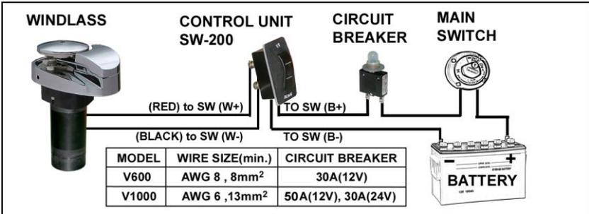
Note: For safety reason, do not connect the power source direct to the battery. Please connect the power cable to the main power switch on your boat.
