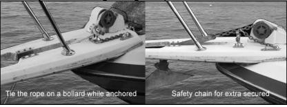
8. The anchor windlass is not designed for continuous operation. Do not use for more than 20 minutes at a time under loading. Allow an interval of 20 – 30 minutes after each operation.
