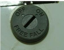
You can set the rotating "free fall" switch(in the right hand side of windlass) by a flat screw driver to be a "on" free fall mode or "off" Power Out mode.
