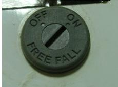
You can set the rotatable "free fall" switch (in the right hand side of windlass) by a flat screw driver to be a "on" free fall mode or "off" Power Out mode.
