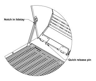
With the quick release pin removed, grasp the lid, pushing back on the center to clear the middle hinge and slide the lid away from the center of the grill until the outer hinge is free of it's pivot pin. Once the lid(s) have been removed they can be washed in warm, soapy water. Installation is reverse of removal.
