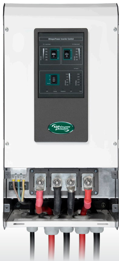
Connection compartment of the AC PowerCube 7 kVA. On the right, double battery connector with 2 x DC PLUS and 2 x DC MINUS connections - one or two separate battery banks can be connected. On the left, the 230 V / 50 Hz output and the connection for the remote control panel and the various set up ports.
